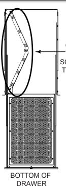
CABLE MANAGEMENT ARM (LEAVE A SERVICE LOOP SO CABLING IS NOT PINCHED) THE ARM CAN BE REVERSED
